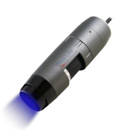
Short Description 1.3 Megapixel resolution Versatility due to exchangeable caps ~375nm + white LEDs 20-220x magnification
