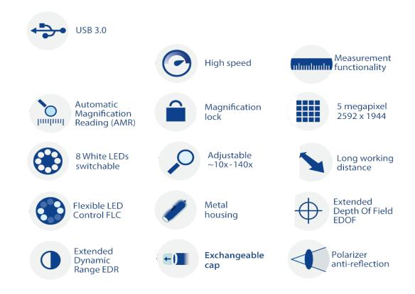
EDOF allows users to automatically capture multiple images at different depths and automatically combine them into one clear image. EDR automatically captures and combines multiple images at different exposure levels to produce a final image with greater dynamic range. The AMR function automatically detects and displays the magnification of the Dino-Lite. The magnification is displayed within the Dino-Lite software and stored with the captured picture and simplifies the measuring process.
