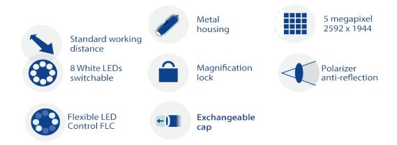
The AM7515MZT is part of the universal range and with its standard working distance and wide magnification range from 10 - 220x, it is suitable for a wide range of applications. Because of the built-in polarization filter this model is ideal when working with shiny or reflective objects such as metal, plastic, glass, jewelry, electronics, etc. The AMR function is of particular importance when the measurement functions are frequently used.
