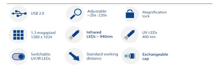
Multiple lighting options provide the ability to view magnified objects under normal external lighting sources such as white light or under near IR, or UV lighting by simply
